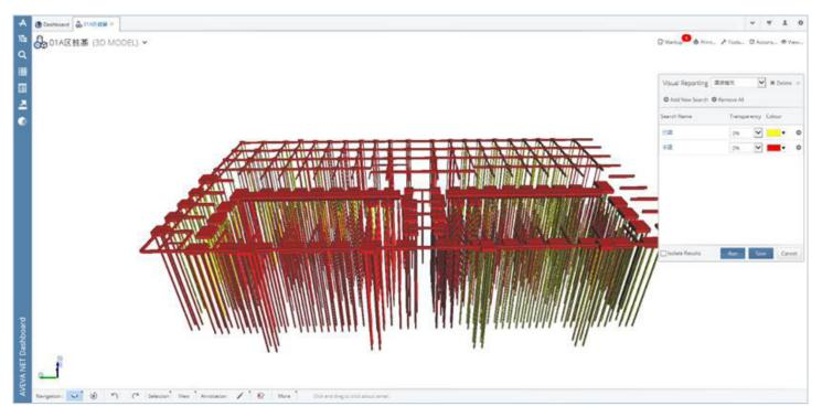
Using AVEVA Asset Information Management, the construction team leader can see the task and the 3D model of the current construction area so that multiple construction teams can quickly understand the tasks they need to complete. (red indicates constructed, yellow indicates to-be-constructed). Source: Shanghai Environmental Laogang Phase II Project Department
