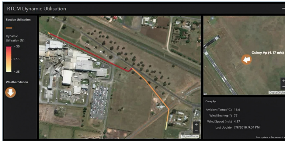
Integration of AVEVA PI System with Esri ArcGIS reveals the dynamic load on a segment of power line in real time. Segments that are more parallel to the direction of the wind retain more heat and have less excess power-carrying capacity than more perpendicular segments.
