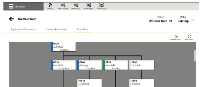
To execute a recipe an operator simply assigns a recipe to equipment and starts, monitors and controls the execution. Parameter values can be adjusted within the defined limits either prior to a recipe start or even prior to a capability being executed.
