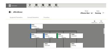
To execute a recipe an operator simply assigns a recipe to equipment and starts, monitors and controls the execution. Parameter values can be adjusted within the defined limits either prior to a recipe start or even prior to a capability being executed.
